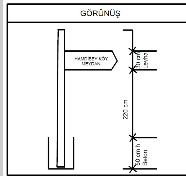
The wooden guidance signboard will be 4 pieces signboards of 30cm width 2 cm thick made on a 10\*10\*220 cm (50 cm will stay within the concrete) impregnated pine timber foot. On the wooden signboard the captions “DUPNISA”, “BALABAN”, “SİSLİOBA” and “İĞNEADA” will be embedded and painted with black paint.
