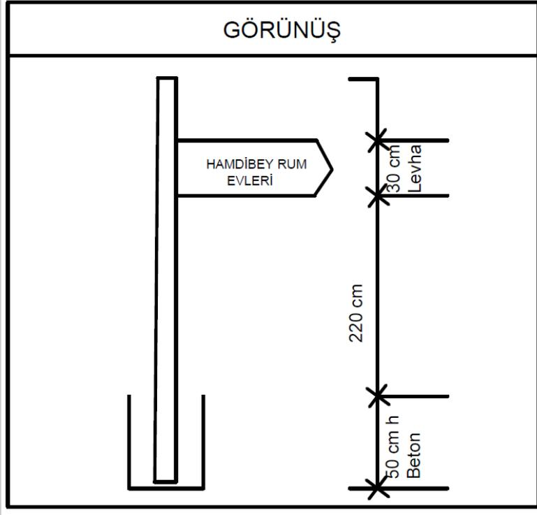
The wooden guidance signboard will be 1 piece signboard of 30cm width 2 cm thick made on a 10\*10\*220 cm (50 cm will stay within the concrete) impregnated pine timber foot. On the wooden signboard the caption “HAMDİBEY VILLAGE” will be embedded and painted with black paint.
