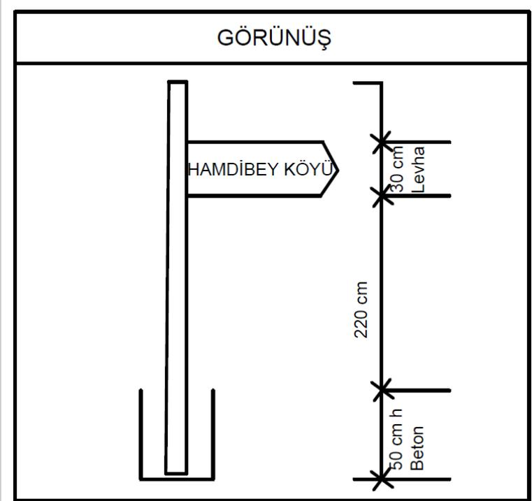
The wooden guidance signboard will be 1 piece signboard of 30cm width 2 cm thick made on a 10\*10\*220 cm (50 cm will stay within the concrete) impregnated pine timber foot. On the wooden signboard the caption “HAMDİBEY VILLAGE SQUARE” will be embedded and painted with black paint.
